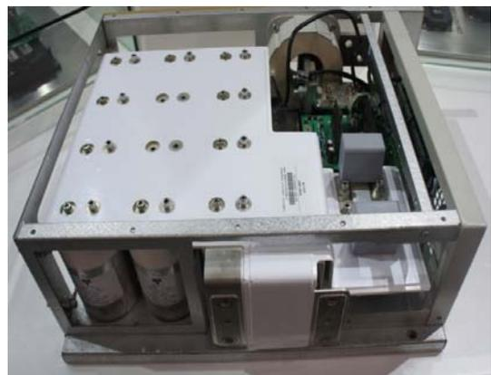
Fig.6 MPDStack™ for renewable energy comprises of half bridge cell
