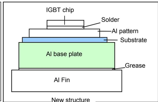
Fig.4 Structure of new MPD IGBT with aluminum baseplate
