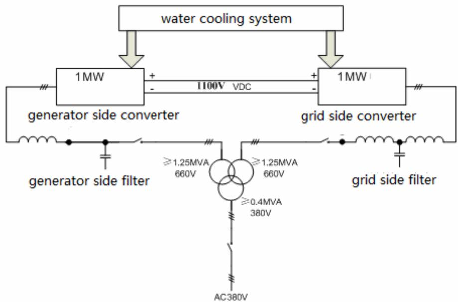
Fig.11 Diagram of power-fed test based on 1MW converter
