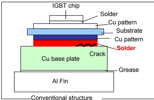
Fig.3 Structure of conventional IGBT with copper baseplate
