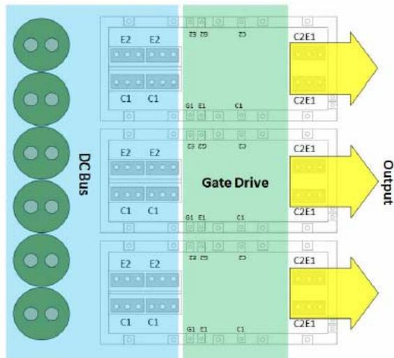
Fig.16 Transparent view of a three phase solar inverter based on 2500A/1200V IGBT
