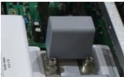
Fig.14 1200V/3.3uF snubber capacitor specified for new MPD IGBT from Vishay
