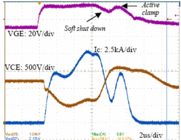
Fig.8 Short circuit test waveform of 1800A/1700V new MPD IGBT module
