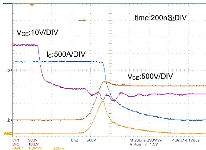
(c) turn-off waveform of CM1800DY-34S
